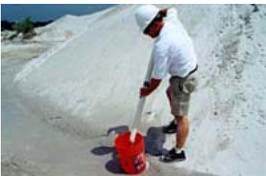
Empty the sample from the tube into a clean, 5-gallon bucket.
