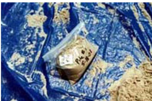
Place the 1-gallon sample into a plastic, zip-lock bag. Label the outside of the bag using a permanent marker. Record the pile number and date of collection. Print the same information on a mailing label and place the label on the outside of the bag. Place the sealed and labeled bag into another plastic bag and seal it with duct tape. This labeling and double-bagging procedure is important to ensure the lab receives the sample intact.
