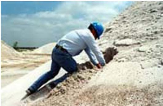
Dig a hole into the face of the pile to prevent collection of any of the sand from the surface of the pile. Expose an undisturbed face of the pile into which the collection tube can be inserted. When you first dig into the pile, material from above will usually flow down the face into the area you are clearing. Keep digging until the hole becomes stable. The shovel also works very well to expose an undisturbed face. Make a vertical cut down into the face just above the sampling point.
