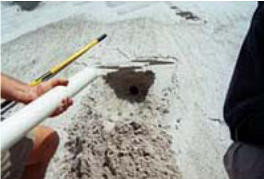
Carefully remove the collection tube from the face of the pile.
